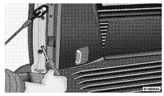
**Removing The Two Screws**
